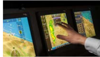
Rockwell Collins' latest configuration of Pro Line Fusion® features the industry's first touch-screen primary flight displays.
